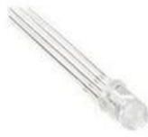
Fig 4: Common cathode RGB LED
